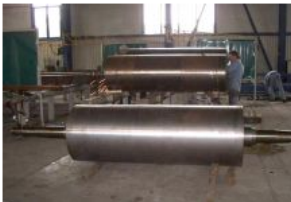
Pulleys for transport conveyors, PP "Kopovi Kostolac", Serbia
